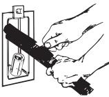
Move washer close to final position. Put "hook" end of drain hose into standpipe. Estimate length of drain hose needed when washer is in final position. Hose must be cut exactly to length so "hook" end is held tightly over edge of standpipe. If drain hose is too long, cut straight end of hose. (Do Not cut "hook" shaped end of drain hose.)
